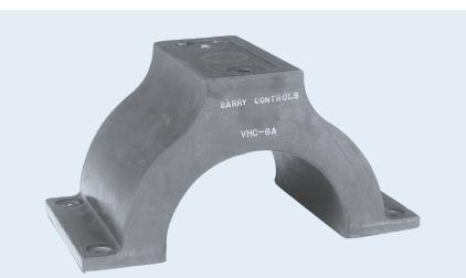
Barry VHC-Series mounts are special purpose, mid-frequency isolators designed to protect sensitive equipment when high level shock and vibration inputs are expected. Typical applications include electronic equipment installed in mobile equipment subjected to off-road environments.
